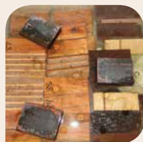
Water-Soak Cycle Test
